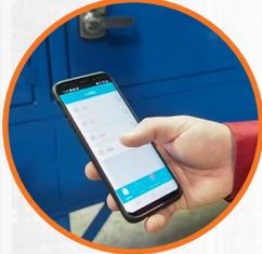
Optional electronic locks can be unlocked onsite by RFID cards or key fobs and can be managed offsite via a secure smartphone app.
